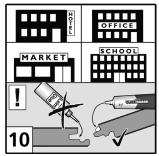
**Preparation:** Please store the packets 48 hours prior to installation under the same climatic conditions (temperature and moisture) as the actual installation process [1]. Important pre-condition for proper fitting and long-term durability of the laminated flooring is a room temperature of ca. 20°C and a relative humidity of around 50 – 70%.
